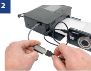
Plug camera USB cable into adapter and into camera.
