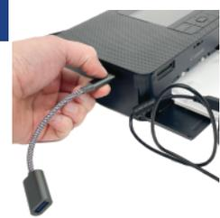
To plug camera into printer, insert a USB-C to USB adapter into printer. (sold separately)
