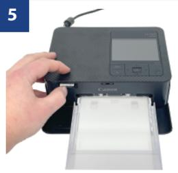
Insert SD card in slot on the front of printer, label side up.
