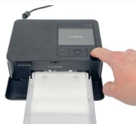
Press power button to turn on the printer.
